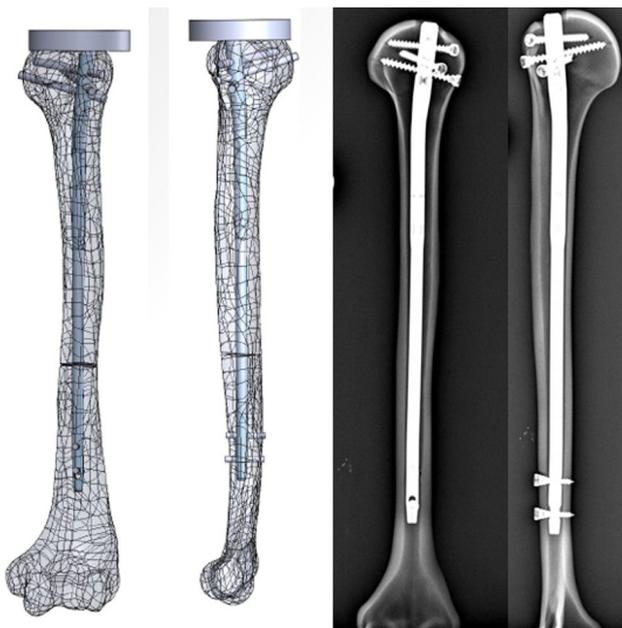
**Fig. 1** Geometric sawbone–Dinamic T Humerus nail model made with the SOLIDWORKS Simulation program (3DS-Dassault System) based on X-rays (AP and lateral view)
